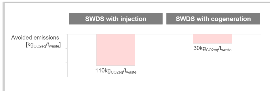
Figure 2 - Comparison of avoided emissions by SWDS equipped with an injection installation and a cogeneration, in the reference mix in 2020, under "good" practices.
