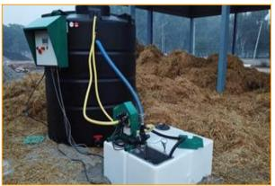
From 150 tonnes of rice straw in a 'batch', expected biogas production will be about 11m3 per hour with a total of around 30,240m3 from each batch.
