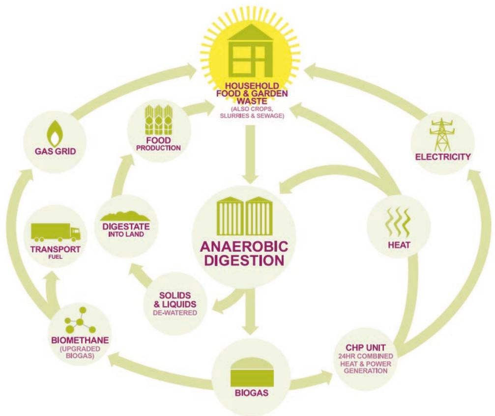
The anaerobic digestion (AD) process
