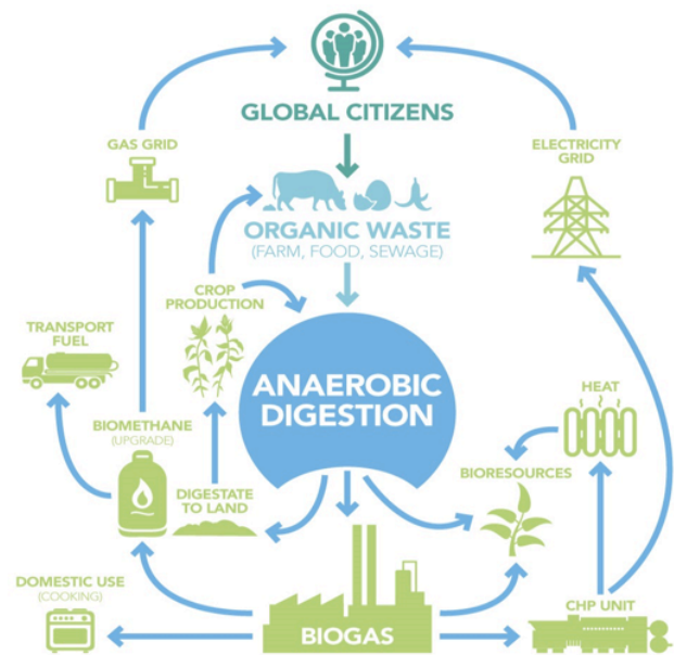
Figure 8: The AD process – inputs, outputs and processes
